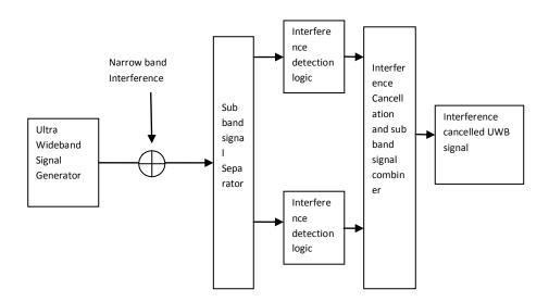
Fig: 14. The Proposed System for Narrowband Interference Detection and Cancellation Logic
