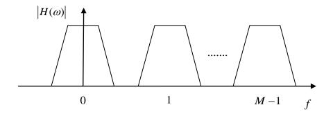
Fig: 2. Sub-Band Splitting of Channel
