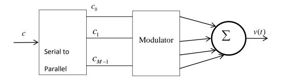
Fig: 1. Multicarrier Modulation Scheme
