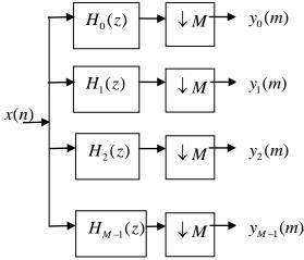
**Fig: 3.** Uniform Decimating M-Channel (Analysis) Filter
