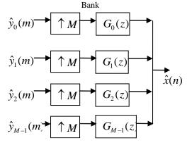
**Fig: 4.** Interpolating M-channel (Synthesis) Filter Bank
