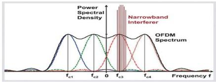
Fig: 10. Narrowband Interference Corrupting OFDM Signal of WLAN 802.11a [16]
