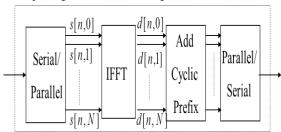
Fig: 6. OFDM Transmitter [12]
