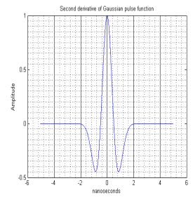
Fig: 12. Second Derivative of Gaussian Pulse Used for UWB Signal Generation
