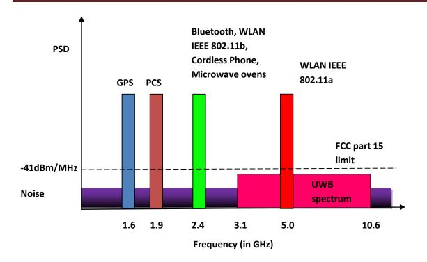
Fig: 5. Spectrum crossover of narrowband interferes in UWB systems [15]
